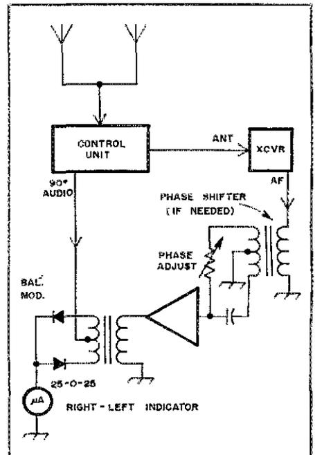
Fig. 8 — Block diagram of a simple right/left indicator. Depending on the setting of the potentiometer, the phase shift may range from 0° to near 180°. In general, one half the full value of resistance of the potentiometer should equal the capacitive reactance of the capacitor at the audio frequency used. Readers with questions should send an s.a.s.e. directly to the author.
