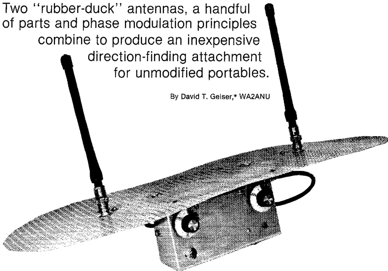
Most amateurs use antennas having pronounced directional effects, either a null or a peak in signal strength, for direction finding. Fm receivers are designed to try to eliminate the effects of amplitude variations and are difficult to use for direction finding without looking at an S meter. Most modern portable transceivers do not have S meters.
